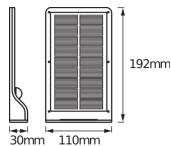
Specifications Ledvance LED Wall Light Doorled Silver 3W - 840 Cool White | Motion and Light Sensor - Solar
