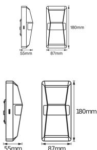
**Specifications Ledvance Endura Pro Wall Light Grey Up & Down - 10W 1000lm - 840 Cool White | IP55 - Motion and Light Sensor**
